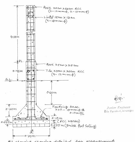
6/5 showing showing detailed box arrangements from foundation to the ceiling (Scarle: - 1:20)
